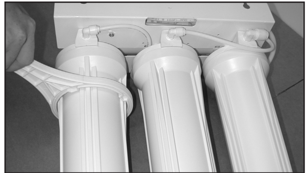
Figure 11 - Using sump wrench to change filter cartridges
